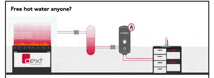
The Dext Heat Recovery system uses innovative splashback panels to capture waste heat. This heat is then used to provide the premises with free hot water and space heating.
